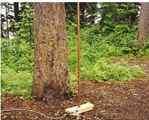
K7ICE/VE7's homebrew 20-meter pipe vertical, complete with ground radials
