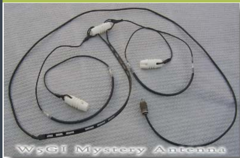
Photo A - Full view of the W5GI multi-band Mystery Antenna with all sections shortened considerably for illustration purposes.
